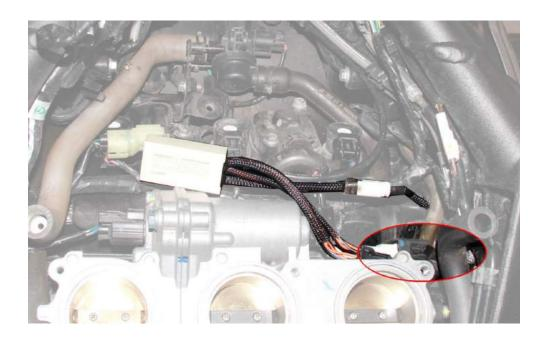
4) Under fuel pump are 2 connectors: for "Gear position sensor" and for "OEM shifting sensor". Disconnect GPS connector (black 4way Sumitomo with wirees in male conector:P, P/B, B/P and B/W) and insert AB wiring harness - 4way natural Sumitomo.
